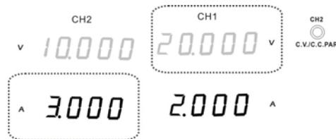
Slave (CH1) voltage level: CH1 meter reading shows the output voltage. In the above case, 20.0V.
